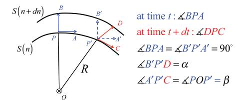
Figure 2: Deformation for a particle traveling from P at time t to P' at time t + dt along a streamline.
