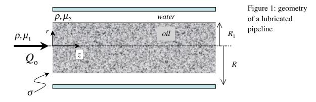
a) Although the oil-water interface shown in the figure above is depicted as planar, in reality under certain operating conditions interfacial waves may form as shown in the picture opposite:
