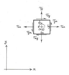
Fig. 5: Illustration of the reason for the stress tensor's symmetry.
