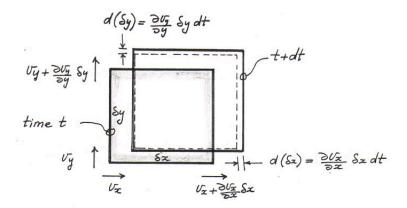
Fig. 11: Linear deformations of a fluid particle.
