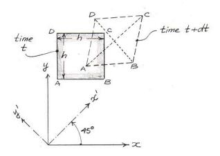
Fig. 8: Why shear and linear deformations are related.
