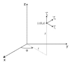
Fig. A.1: Cylindrical coordinate system
