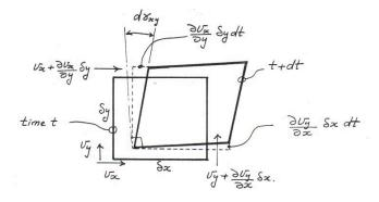
Fig. 7: Shear deformations in a fluid particle.
