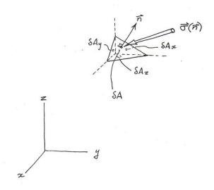
Fig. 4: Tetrahedron-shaped fluid particle at (x, y, z).
