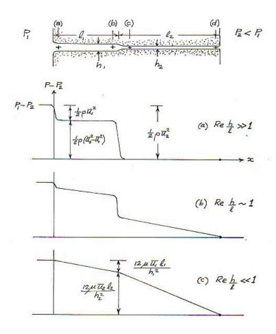
Fig. 2: Pressure distribution under (a) inertia-dominated, (b) intermediate and (c) highly viscous (locally fully developed) conditions.
