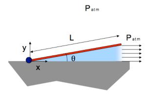
A flat plate is hinged at one side to the floor, as shown, and held at a small angle  $\theta_0$  ( $\theta_0 \ll 1$ ) relative to the floor. The entire system is submerged in a liquid of density  $\rho$ . At t = 0, a vertical force is applied and adjusted continually so that it produces a constant rate of decrease of the plate angle  $\theta$ .
