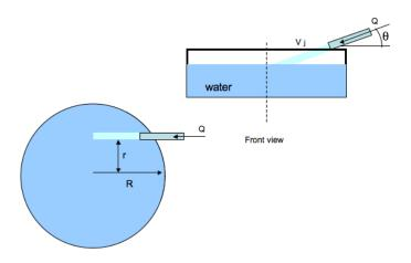
At t = 0, a circular tank of radius R contains water at rest, with a depth h. Between  $0 < t < \tau$ , a water hose is sprayed onto the surface of the water in the tank at a volume flow rate Q and an exit velocity  $V_j$ . The jet impacts tangentially on the water at a radius  $R_j$ , with an angle  $\theta$  relative t the horizontal.
