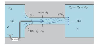
The device connected between compartments A and B is a simplified version of a jet pump. A jet pump, or ejector, is a simplified device which uses a small, very high-speed jet with relatively low volume flow rate to move fluid at much larger volume flow rates against a pressure differential  $\Delta p$  (see the figure).
