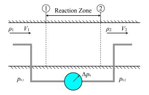
The sketch shows a liquid emulsion (a finely-divided mixture of two liquids) of mean density  $\rho_1$  entering a reaction zone of a constant-area reactor with speed  $V_1$ . The components of the emulsion react chemically, and leave the reaction zone as a liquid at the density  $\rho_2$ . Pitot tubes are installed upstream of the reaction zone. (Pressure inside a pitot tube is stagnation pressure,  $p_0 = p + \frac{1}{2}\rho V^2$ ).
