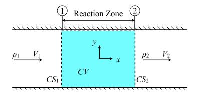
Taking the reaction zone as our control volume, and noting that the cross-sectional area of the reactor is constant, we find from our integral mass conservation relation that
