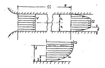
Consider the two-dimensional, incompressible, steady flow of a fluid of constant viscosity in the entrance region of a <u>slit</u> of width 2h. The flow enters the tube (x = 0) with the uniform velocity V. At distance x from the entrance, the boundary layer thickness is  $\delta$ , and the core flow has the speed U. The boundary layer is laminar.
