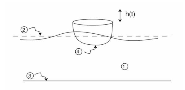
Figure 1. Boundary conditions for the total potential must be met at three places: sea floor (3), free surface (2), structure surface (4). The continuity equation must be satisfied within the fluid (1).
