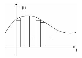
Figure 3. A function f(t) represented as a sum of scaled and time -shifted impulses.
