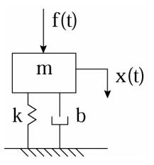
Figure 6. Mass-spring-dashpot system
