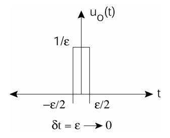
Figure 2. Delta (impulse) function with height 1/e between times -e/2 and e/2 as dt = e goes to zero.
