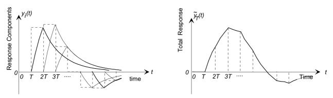
Figure 4: System response to individual pulses in the staircase approximation to u(t).
