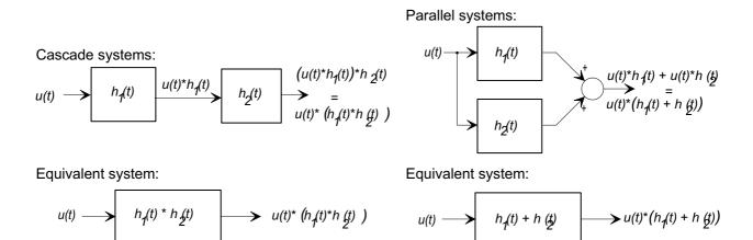
Figure 7: Impulse response of series and parallel connected systems.
