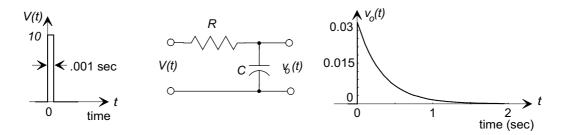
Figure 6: An *RC* filter and its impulse response.
