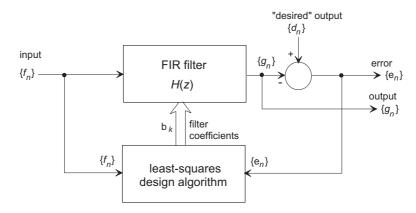
Given an input sequence  $\{f_n\}$ , and a "desired" filtered output sequence  $\{d_n\}$ , the task is to design a FIR filter
