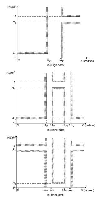
The critical frequencies used in the design are as shown above. For band-pass and band-stop filters it is convenient to define a center frequency  $\Omega_o$  as the geometric mean of the pass-pand
