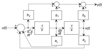
This basic structure may be used to realize the four basic filter types by appropriate choice of the numerator.
