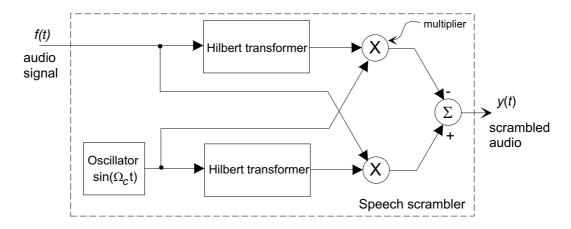
Internally an oscillator generates a constant frequency sinusoid  $\sin(\Omega_c t)$ . Assume for now that the audio signal is a sinusoidal waveform  $A\sin(\Omega_1 t)$ . Determine the output of the system y(t).
