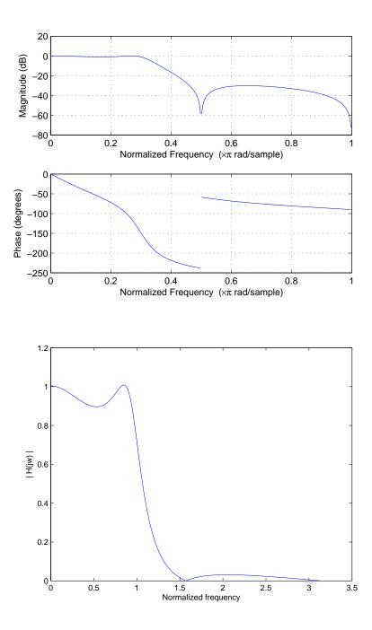
The pole-aero plot shows zeros on the unit-circle at angles  $\Omega = \pi/2$  and  $\pi$ , indicating that the frequency response magnitude should dip to zero at these frequencies. This is seen on the frequency response plots. There are three poles, not on the unit-circle, but in the lowfrequency region, indicating a low-pass action. Note the ripple in the pass-band and the stop-band - a characteristic of elliptic filters.
