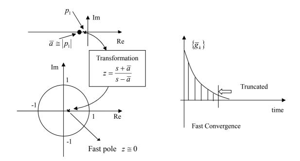
When the original transfer function has many poles, the Laguerre pole is placed near the dominant pole so that most of the slow poles may be approximated by the Laguerre pole.
