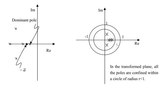
With the bilinear transform, these slow poles are transferred to the ones near the origin of the z-plane. They are fast, hence the transfer function can be approximated to a low order model.
