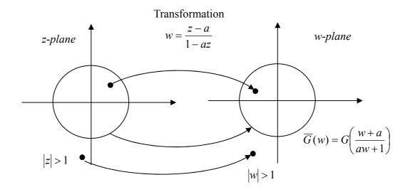
$$\overline{G}(w) = G\left(\frac{w+a}{aw+1}\right) \text{ is analytic in } |w| > 1, \text{ and is proper } G(\infty) = 0$$
