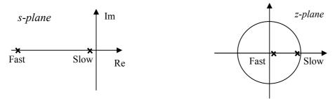
Choose  $\overline{a}$  such that  $p_1 \cong -\overline{a}$ , where  $p_1$  is a slow, stable pole. Using the bilinear transform, this slow pole in the s-plane can be transferred to a fast pole in the z-plane, as shown below. Representing in the z-plane, the transfer function can be truncated; just a few terms can approximate the impulse response since it converges quickly.
