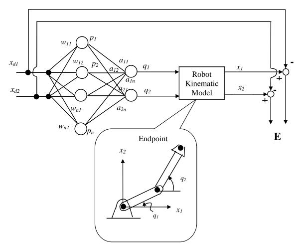
Consider a two degree-of-freedom robot, as shown in the figure below.
