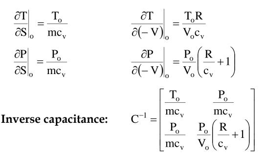
equality of the off-diagonal terms (the crossed partial derivatives) is established using  $P_oV_o = mRT_o$
