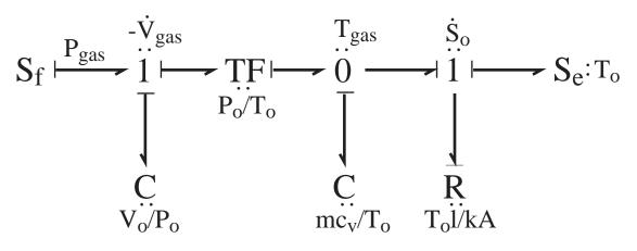
Note the sign change on the capacitor thermal port (to avoid a superfluous 0-junction)
