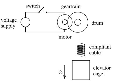
Even more important, the peak stress in the cable is almost double the steadystate stress required to support the weight of the cable.
