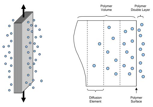
Figure 3: Reticulation of Thin-Film Polymer into Diffusion Elements
