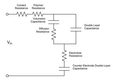
Figure 1: Basic Structure of EAP Electrochemical Circuit
