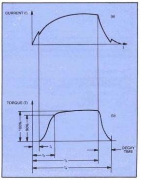
Figure 2. Response and decay time of a typical unit.
