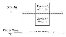
The sketch shows a highly simplified diagram of a dry-dock used in ship maintenance. Once the ship enters the dock, water is drained out by positive-displacements pumps, an operation termed "pumping down the dock". When work is complete, a gate to the harbor admits water, an operation termed "floating the dock". Your task is to model the heavemode oscillatory behavior (i.e. vertical motion only) of a ship in the dock.
