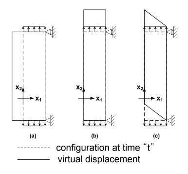
Figure 1. Three simple independent virtual displacement patterns.
