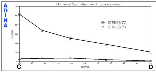
Figure 3. Stresses on the horizontal symmetry line solved using 4-node elements
