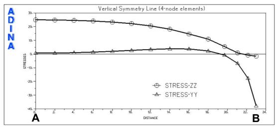
Figure 5. Stresses on the vertical symmetry line solved using 4-node elements
