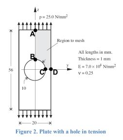
In this solution, the horizontal symmetry line corresponds to the line CD and the vertical symmetry line corresponds to the line AB. The distance of the horizontal line is measured from the point C and the distance of the vertical line is measured from the point A. (See Figure 2.)
