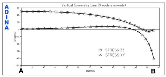
Figure 6. Stresses on the vertical symmetry line solved using 9-node elements
