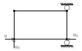
The clamp for  $u_5$  "sees" no more stiffness. A rigid body rotation is possible. Therefore there will be a zero diagonal term after the third step of Gauss elimination.
