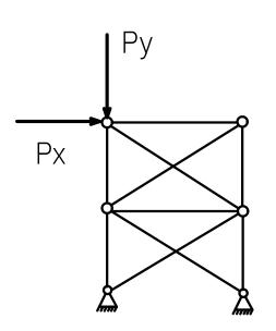
suppose we were to analyze this pin-jointed structure
