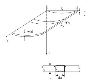
strain in y constrained by adjacent plate anticlastic curvature  $R_V = 1/v * R$
