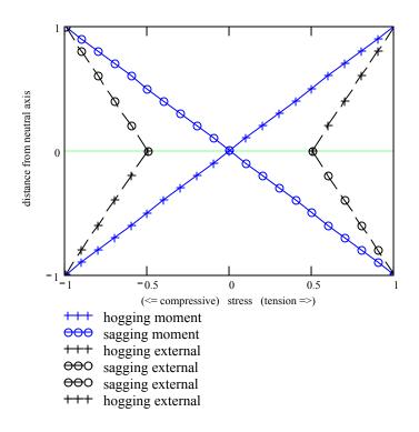
first set tension at neutral axis at half the maximum in tension and compression ;
