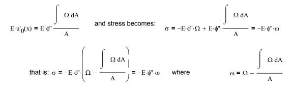
this defines the *normalized* coordinate in the same sense as y and Y etc. as an aside:  $u' = -\phi' \cdot \omega$  =>  $u = -\phi' \cdot \omega + constant$   $d\omega = h_D \cdot ds$ in this sense,  $\omega$  is defined as the unit warping function
