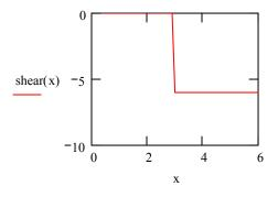
as above total shear along beam with ll := 0 and ul := 4 => shear  $(x) := \sum_{i=ll}^{ul} f_i \cdot (x \ge xx_l)$
