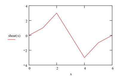
for later comparison, let's rename this  $shear_1(x) := shear(x)$ note that shear curve starts and ends at 0; why??
