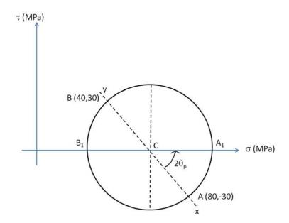
The center, C, is located at (40 + 80)/2 = 60 MPa on the  $\sigma$  axis.
