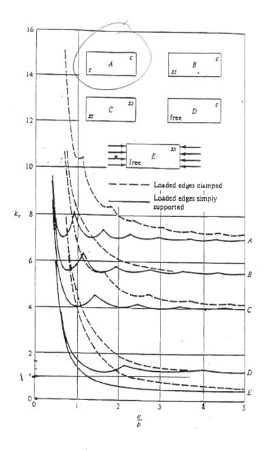
We are considering case D, a/b = 5. Notice that the cases for the loaded edges being clamped and simply supported are almost overlapping in buckling coefficients  $K_c = 1.3$
