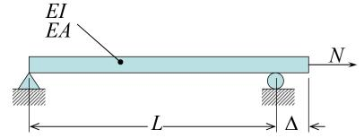
a) Calculate the maximum allowable midspan deflection  $(w_o)_{critical}$  under which the beam will slide off its support.
