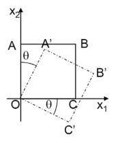
Only **rigid body rotation** in this case, there should be 0 strain everywhere Deformation
