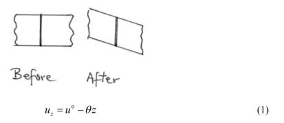
where  $u^{\circ}$  is the displacement of the beam axis
