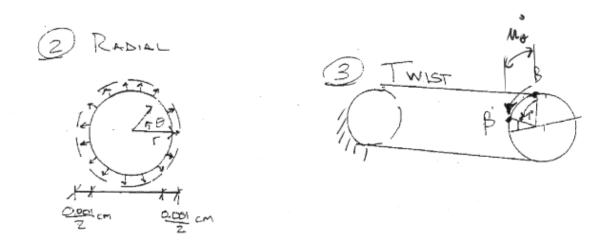
Evaluate deformation components at the end cross-section
