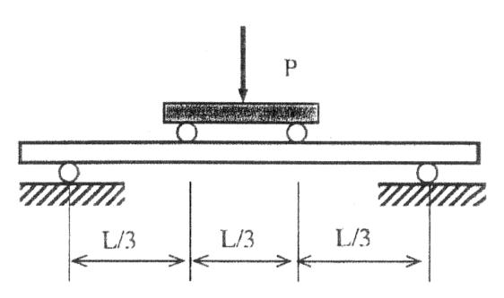
Consider the four –point bending of a beam of length L. The beam is loaded by two rollers parted by a distance of L/3. The material of the beam is rigid, perfectly plastic. Determine the load capacity of the beam under two different end conditions.
