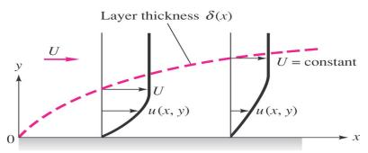
A reasonable approximation for the two-dimensional incompressible laminar boundary layer on the flat surface is
