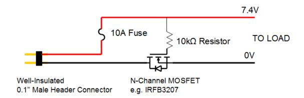
The MOSFET (a type of transistor) only turns on if the current passing through the resistor is positive. It needs to be a sizeable MOSFET, rated for much more than 10A. Some will be made available in lab
