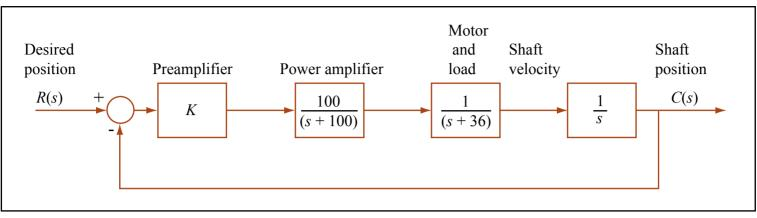
**Specification:** 9.5% overshoot. For 9.5% overshoot, the required damping ratio is  $\zeta = 0.6$ . Using the damping ratio–phase margin relationship, we find
