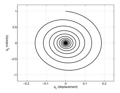
The impulse responses  $q_1(t) \equiv x_1(t), q_2(t) \equiv v_1(t)$ . are again plotted below sideby-side:
