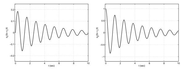
We leave the overdamped case for you to ponder. Some thought should convince you that the Phase Space diagram would then look like a curved line, simpler than a spiral, but still converging to the origin  $\mathbf{q} = (0 \ 0)^t$  as  $t \to \infty$ . You can also verify your conclusion in MATLAB by using the tf command to define an overdamped transfer function of your choice and then the impulse command to generate its impulse response.
