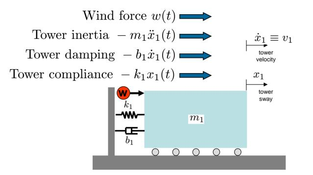
Force balance:  $w(t) - m_1 \ddot{x}_1(t) - b_1 \dot{x}_1(t) - k_1 x_1(t) = 0 \Rightarrow$
