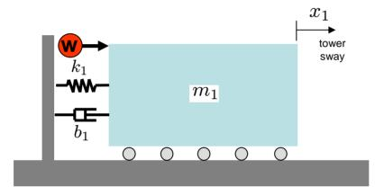
We begin by considering the tower by itself, i.e., without the slider-spring-damper compensation system.
