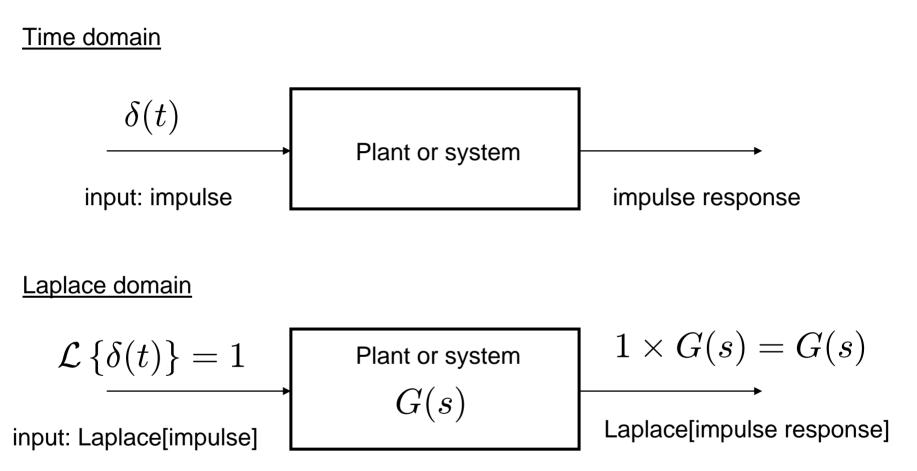
The Laplace transform of the impulse response is the Laplace transform of the transfer function
