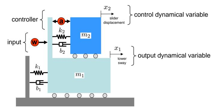
The objective of control is to *minimize the output* (tower sway) subject to an *impulse input* (wind force)
