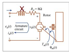
KVL around the DC motor circuit loop (neglecting the inductance  $L_a$ ) yields
