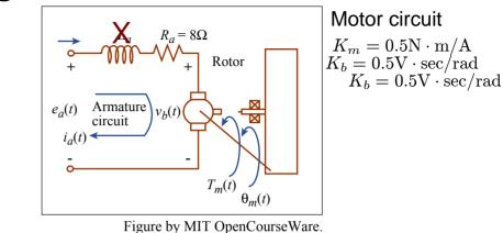
Case study: motor with gear load
