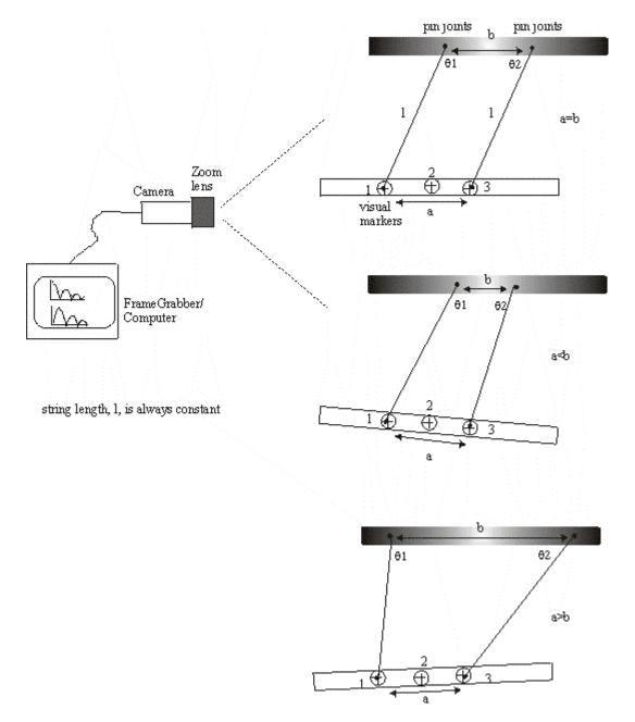
Task 0: Locate the center of mass (CM) of the rod. How would you find it? Place a visual marker at the CM.
