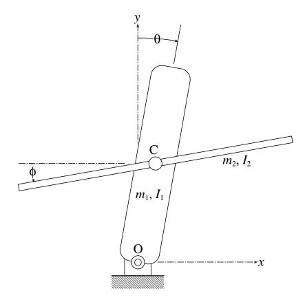
Figure 4: Mechanical model of tight-rope walker.
