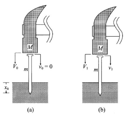
(a) The initial momentum of the hammerhead is  $MV_0$  in the downward direction and the combined downward momentum of the hammer and the nail, after the impact, is
