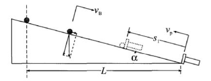
Let distance up the slope be denoted by s. The piston starts at s = 0 with constant velocity  $v_p$ . The displacement of the piston at time t, before it hits the ball, is
