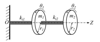
Two disks of radius  $r_1$  and  $r_2$  and mass  $m_1$  and  $m_2$  are mounted in series with steel shafts. The shaft between the base and  $m_1$  has length  $L_1$  and the shaft from  $m_1$  to  $m_2$  has length  $L_2$ . The shafts have cross section polar moments of inertia,  $J_{zz1}$  and  $J_{zz2}$ . They also have shear moduli,  $G_1$  and  $G_2$ . The torsional spring constant of each
