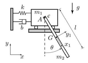
The linearized equations of motion for the system are the same as found in problem set 10 except that an external torque,  $-c\dot{\theta}$ , resulting from the linear damper at the pivot must be included in Equation 2 below, the rotational equation of motion:
