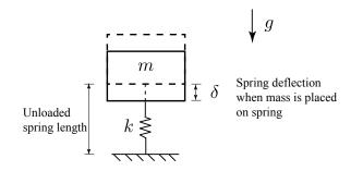
When a mass is placed on the spring, in the presence of gravity, the spring deflects due to the mass's weight.
