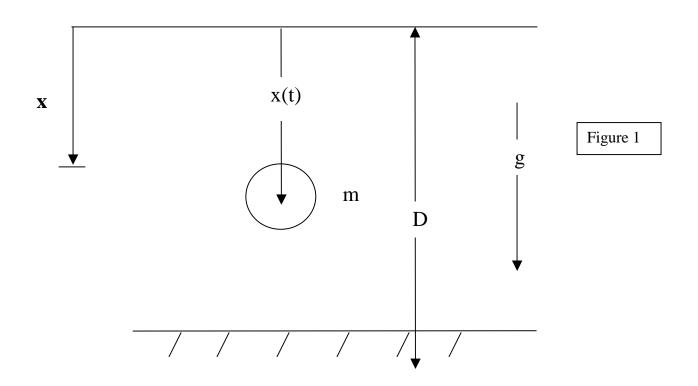
A rigid hollow negatively buoyant sphere of mass *m* with frontal area *A* and volume *V* is given an initial downward velocity  $v_i$  at the surface of the ocean of depth *D* and water density  $\rho_w$ . The fluid force on the sphere is given by
