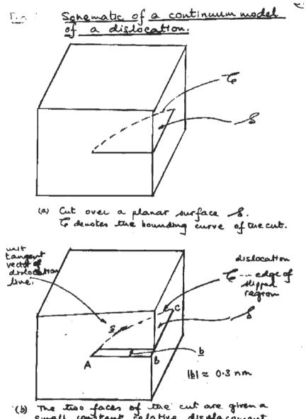
(b) The two faces of the cut are given a small constant relative displacement & equal to a lattice sector and the faces of the cut are welded together. **Plastic Shear Strain Increment**
