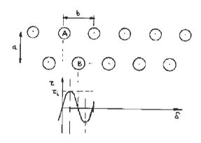
$$au = au_i \sin\left(2\pi \frac{\delta}{b}\right), \quad au = au_i \left(2\pi \frac{\delta}{b}\right), \quad \frac{\delta}{b} \ll 1$$
