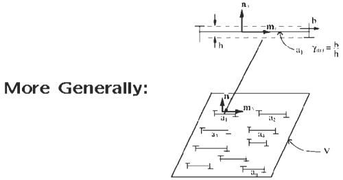
$$v_{\text{slip}} = h \times \sum_{k=1}^{n} a_k, \qquad \gamma_{\text{tr}} = \frac{b}{h}$$
