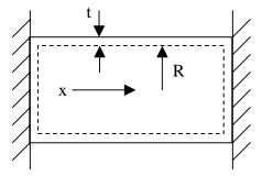
1) The internal pressure in the tank is brought to a value p. Obtain expressions for the resulting displacement of the plate  $u_c$ , and for the change in tank wall thickness  $\delta_t$ . What is the radial strain in the tank wall? What is the circumferential strain in the tank wall?
