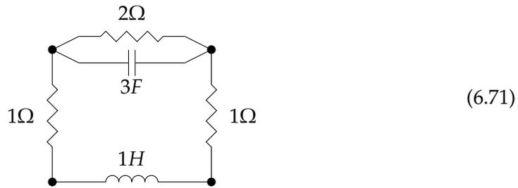
We might formally consider this as a graph on the set of four ports, where each edge is labeled by a type of circuit component (for example, the top edge would be labeled as a resistor of resistance  $2\Omega$ ). For this circuit to be a morphism in some category, i.e. in order to allow for interconnection, we must equip the circuit with some notion of interface. We do this by marking the ports in the interface using functions from finite sets:
