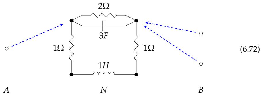
Let  $N$  be the set of nodes of the circuit. Here the finite sets  $A$ ,  $B$ , and  $N$  are sets consisting of one, two, and four elements respectively, drawn as points, and the values of the functions  $A \rightarrow N$  and  $B \rightarrow N$  are indicated by the grey arrows. This forms a cospan in the category of finite sets, for which the apex set  $N$  has been *decorated* by our given circuit.
