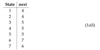
We call the schema **DDS** to stand for discrete dynamical system. Indeed, we may think of the data in the **DDS**-instance of Eq. (3.65) as listing the states and movements of a deterministic machine: at every point in time the machine is in one of the listed states, and given the machine in one of the states, in the next instant it moves to a uniquely determined next state.
